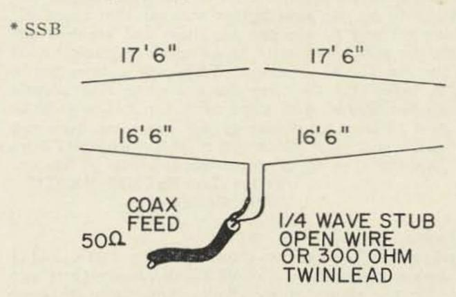
2 ½ waves in phase driven elements 2 refectors (one behind each driven element)
